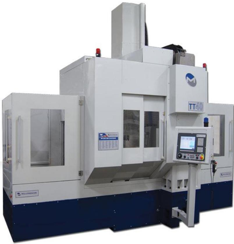
The NEW MILLTRONICS TT40 is a new concept to keep your CNC operator busy every moment. This rigid cast iron bridge construction machine is unique, with dual tables (1015 x 1100mm) and dual ball screws. With 30m/min rapids it is designed for high production and high swarf removal. Travels 1066 x 1016 x 735, spindle 50-10,000 rpm, weight 18,000kgs ( Larger model available) ..... P.O.A
